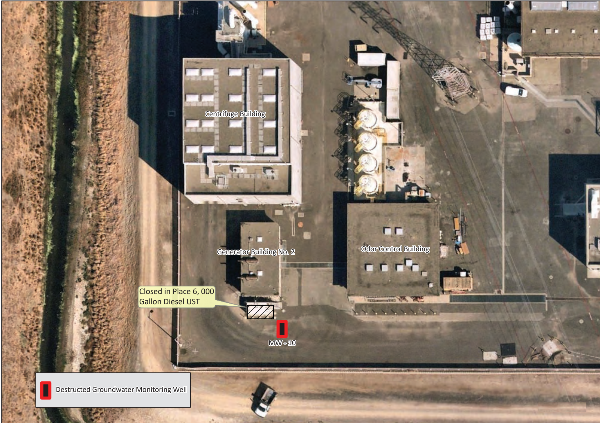
68 of 96 Figure 4: Closed-in-Place 6,000 Gallon Diesel UST
